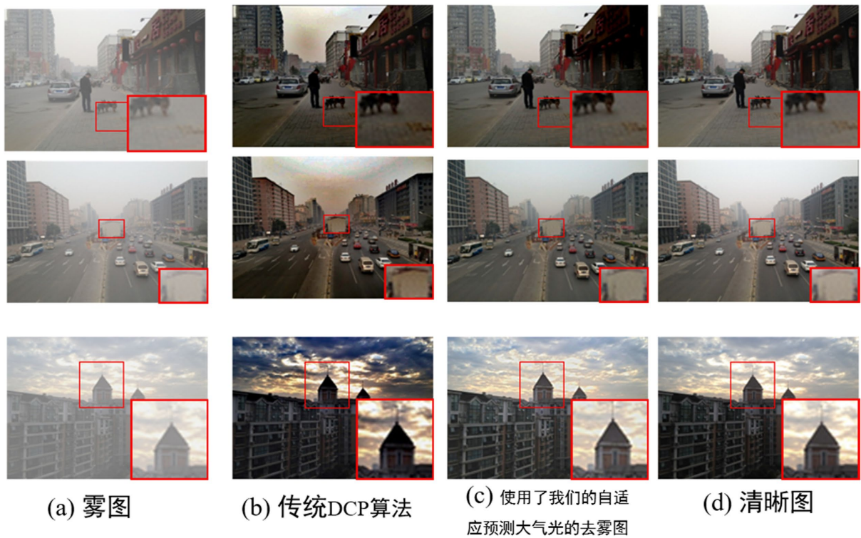
Figure 2. Visual comparison of the proposed adaptive atmospheric light prediction method and the traditional DCP method on the SOTS-outdoor and HSTS datasets
