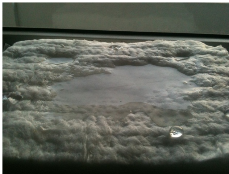
Figure 5. The surface of magnesium silicate fiber blanket is sprayed with water
