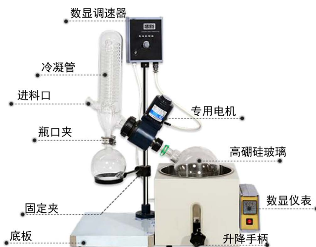
Figure 2. Rotary evaporator (Model: RE-5001) 图 2. 旋转蒸发仪(型号: RE-5001)
