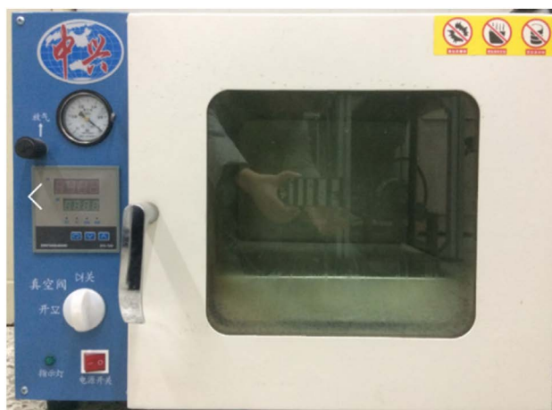
Figure 4. Vacuum drying oven (Model: DZF-6020A) 图 4. 真空干燥箱(型号：DZF-6020A)
