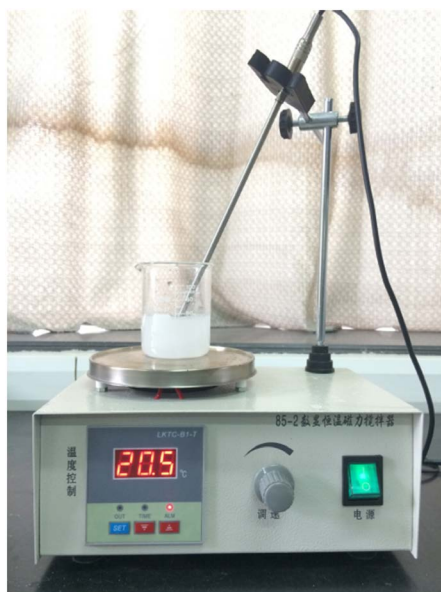
Figure 3. Thermostatic magnetic stirrer (Model: 85-2) 图 3. 恒温磁力搅拌器(型号：85-2)
