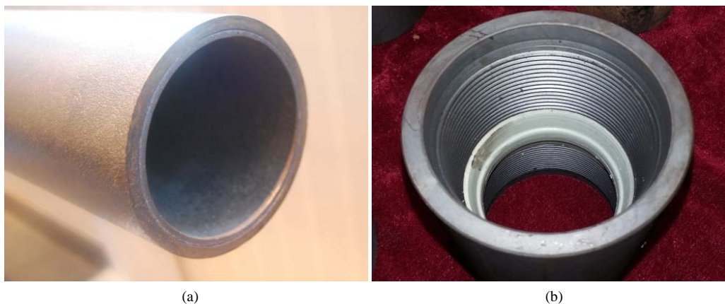
Figure 3. The end of ceramic lined oil pipe and non-metallic protection of coupling. (a) The end of ceramic lined oil pipe; (b) Non-metallic protection ring of coupling 图 3. 陶瓷内衬油管端面与内嵌非金属保护环的接箍图。(a) 陶瓷内衬油管端面图；(b) 带内嵌非金属保护环的接箍图
