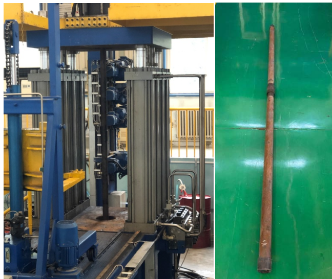
Figure 5. Ceramic lined tubing specimen and full scale tensile 图 5. 陶瓷内衬油管试样与全尺寸拉伸图示
