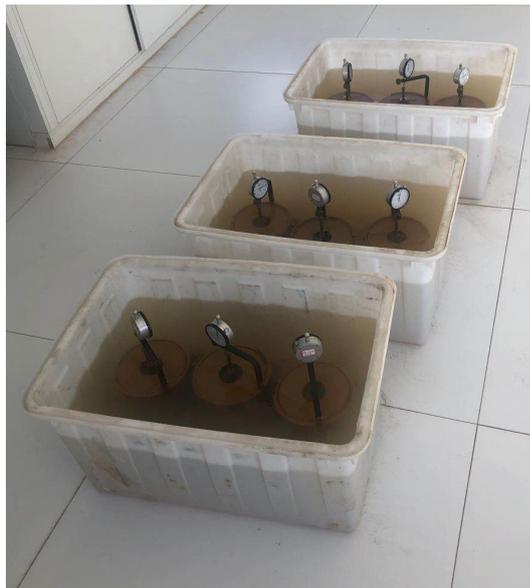
**Figure 2.** The soaking process of the specimen
