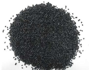
Figure 2. Graphene nanosheets coated with polypropylene masterbatches
