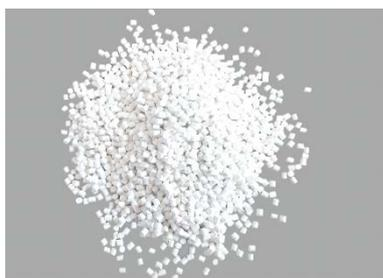
Figure 1. Polypropylene masterbatch
