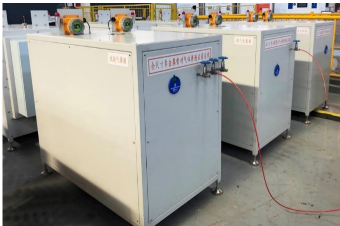
Figure 1. Test instrument for gas permeability resistance of full size non-metallic pipe
