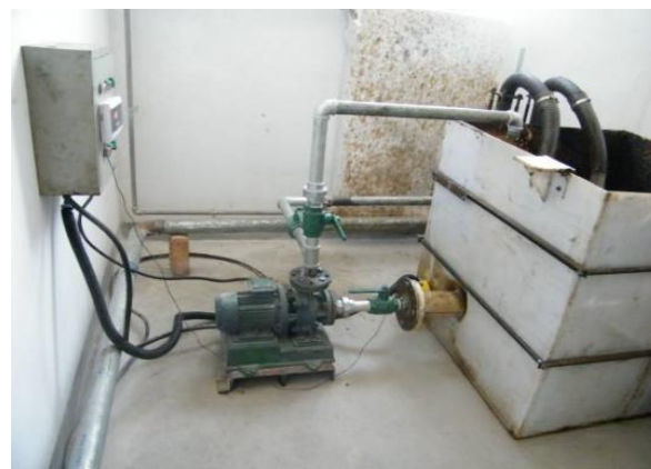
Figure 5. Test instrument for anti-scaling and wax deposition performance of non-metallic pipe 图 5. 非金属管抗结垢结蜡性能试验装备
