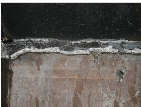
**Photo 7.** Condition of the horizontal sealant after the test
