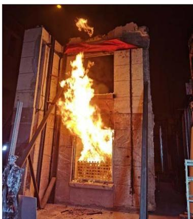
**Photo 3.** The flame spread to the upper part of the second layer window (at the beginning of the test for 3 minutes)
