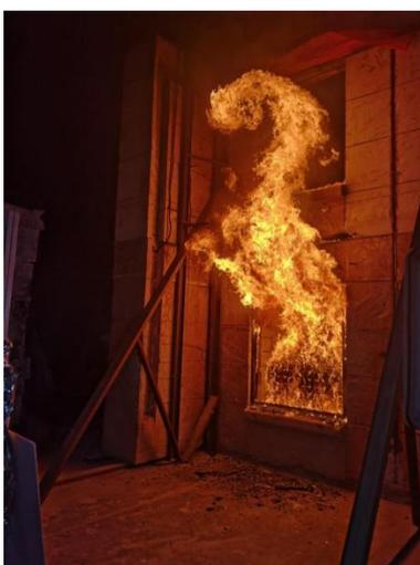
**Photo 4.** Flashover (at the beginning of the test for 8 minutes)
