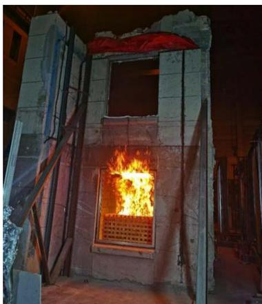
**Photo 2.** The wooden crib fire burned to the upper part of the first floor window (at the beginning of the test for 45 seconds)
