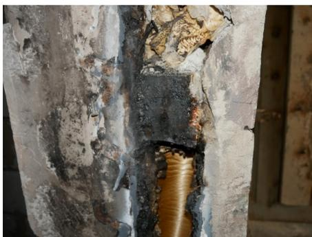
**Photo 6.** Condition of the window wooden brick after the test
