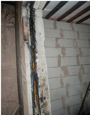
**Photo 5.** Condition of insulation material on the left side of the window after the test
