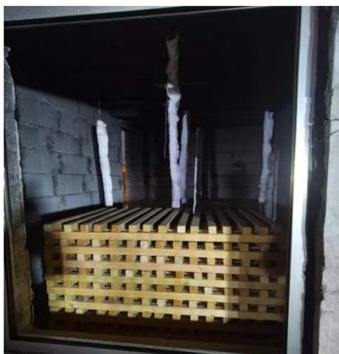
Photo 1. The placement of combustibles in the fire room before the test
