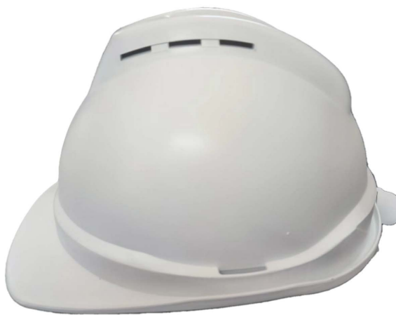
Figure 1. Safety helmet with passive radiative cooling coating
