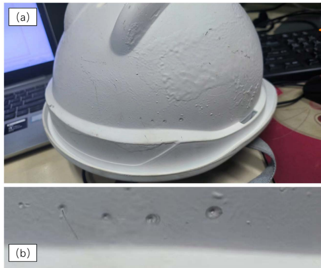
Figure 4. Result of the puncture resistance test 图 4. 抗穿刺强度测试结果
