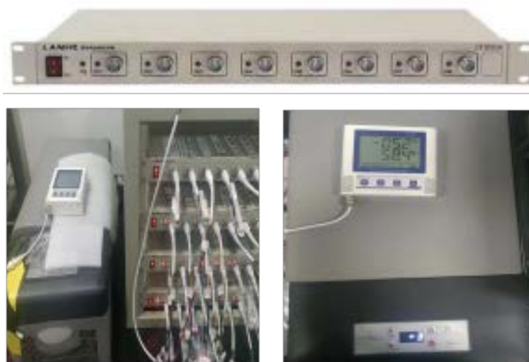
Figure 6. Low temperature battery charging and discharging, low-temperature heating battery charging and discharging LANDIAN cycle testing device 图 6. 低温电池充放电、低温加热电池充放电 LANDIAN 循环测试装置
