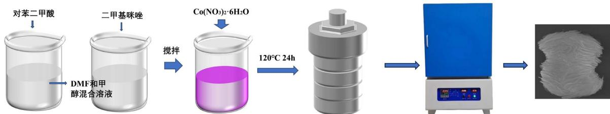
**Figure 1.** Schematic diagram of double ligand Co-MOF synthesis
