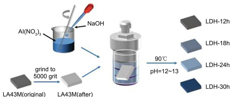
Figure 4. Hydrothermal operation process [13]
