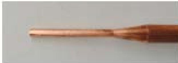
**Figure 7.** Schematic diagram of copper tube after diameter reduction
