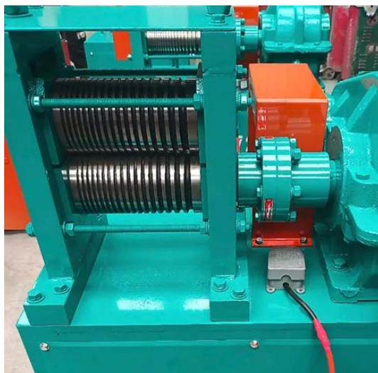
Figure 1. Schematic diagram of roller pointing machine structure
