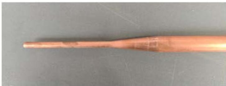
Figure 20. Schematic diagram of pointing zone appearance
