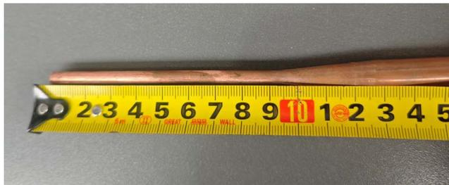
Figure 15. Schematic diagram of actual pointing length
