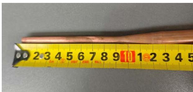
Figure 17. Measurement diagram of straight section and transition section in pointing zone
