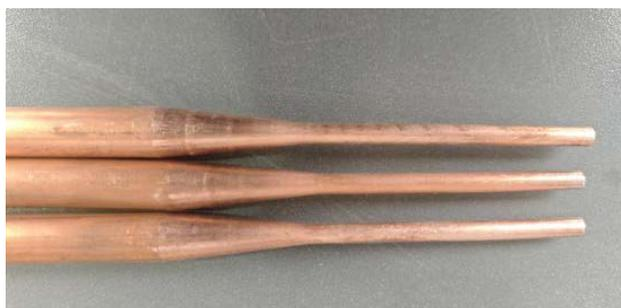
Figure 16. Schematic diagram of post-pointing appearance
