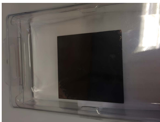
Figure 1. Copper plate with composite coating 图 1. 具有复合涂层的铜板
