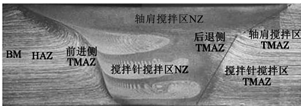
Figure 2. Microstructure morphology of the friction stir welded aluminum alloy joint 图 2. 铝合金经过搅拌摩擦焊接后接头的组织形貌图
