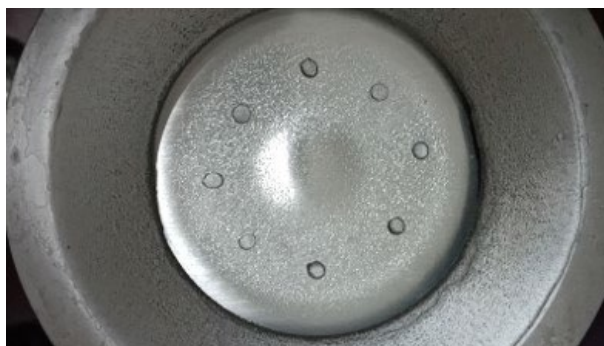
Figure 1. Schematic diagram of the symmetrical placement of the sputtering ring area of the Pt disc on the \text{Ni}_{80}\text{Fe}_{20} alloy target 图 1. Pt 圆片在 \text{Ni}_{80}\text{Fe}_{20} 合金靶上溅射圆环区域对称摆放的示意图
