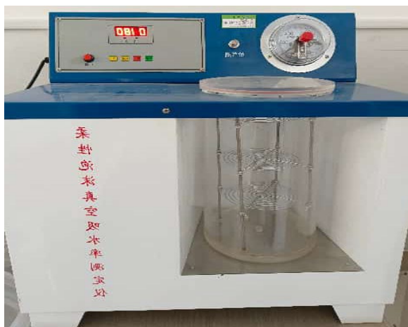
Figure 3. Flexible foam vacuum water absorption tester 图 3. 柔性泡沫真空吸水率测定仪
