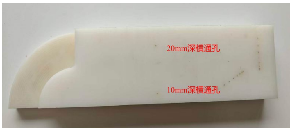
Figure 1. CSK-IA standard reference block made of polyethylene 图 1. 聚乙烯 CSK-IA 标准试块
