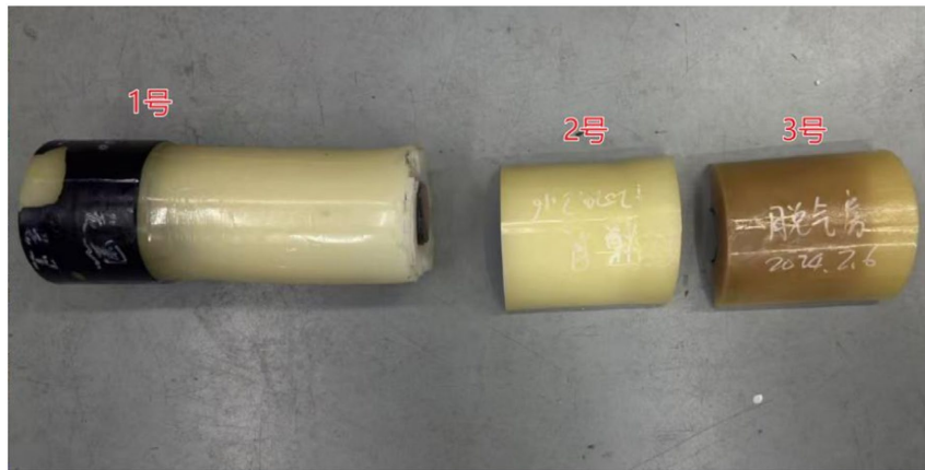
Figure 3. XLPE submarine cable joint containing natural defects 图 3. 含真实缺陷的交联聚乙烯海缆接头
