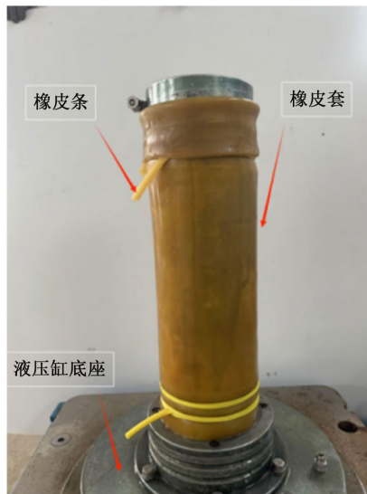
Figure 4. Installation of triaxial specimen 图 4. 三轴试件安装
