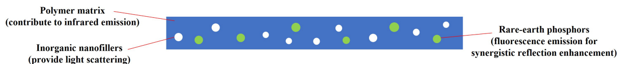
Figure 2. Schematic diagram of single-layer radiative cooling materials based on rare-earth phosphor photoluminescence 图 2. 单层结构稀土荧光粉光致发光辐射制冷材料示意图
