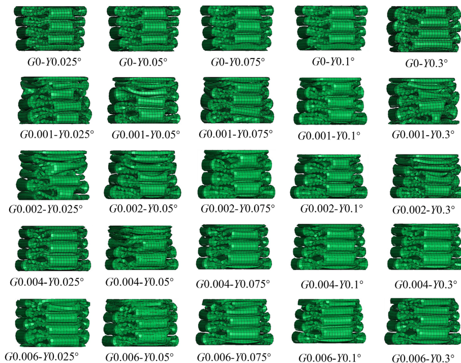
Figure 10. Final deformation modes of thin-walled tubes with torsional initial geometric imperfections 图 10. 扭转型初始几何缺陷下薄壁管的最终变形模式
