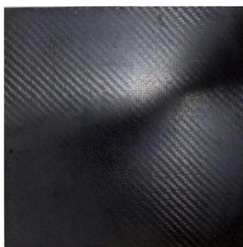
Figure 1. Photograph of a polyimide composite panel 图 1. 聚酰亚胺复合材料平板照片
