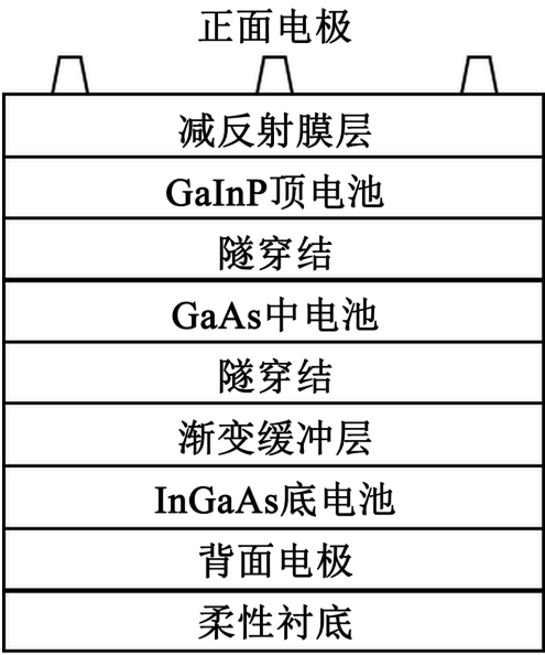
Figure 1. Structure diagram of the triple-junction flexible GaAs solar cell chip
