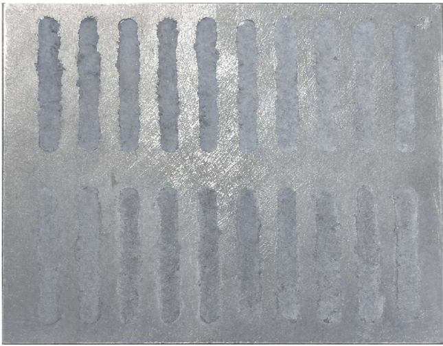
Figure 1. Macroscopic morphology of alloy powder preset in grooves on the Q235 steel substrate 图 1. Q235 钢基体表面凹槽内预置合金粉末的宏观形貌
