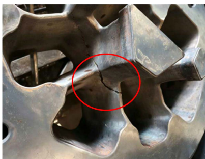
Figure 1. Cracking of large-sized hot extrusion dies
