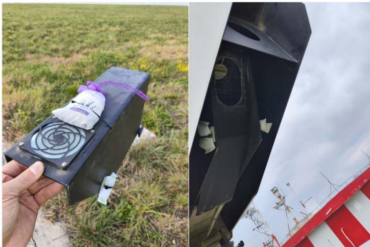
**Figure 4.** Placement of camphor balls (with the TR30 window inner cover on the left and the outer cover on the right after placement)
