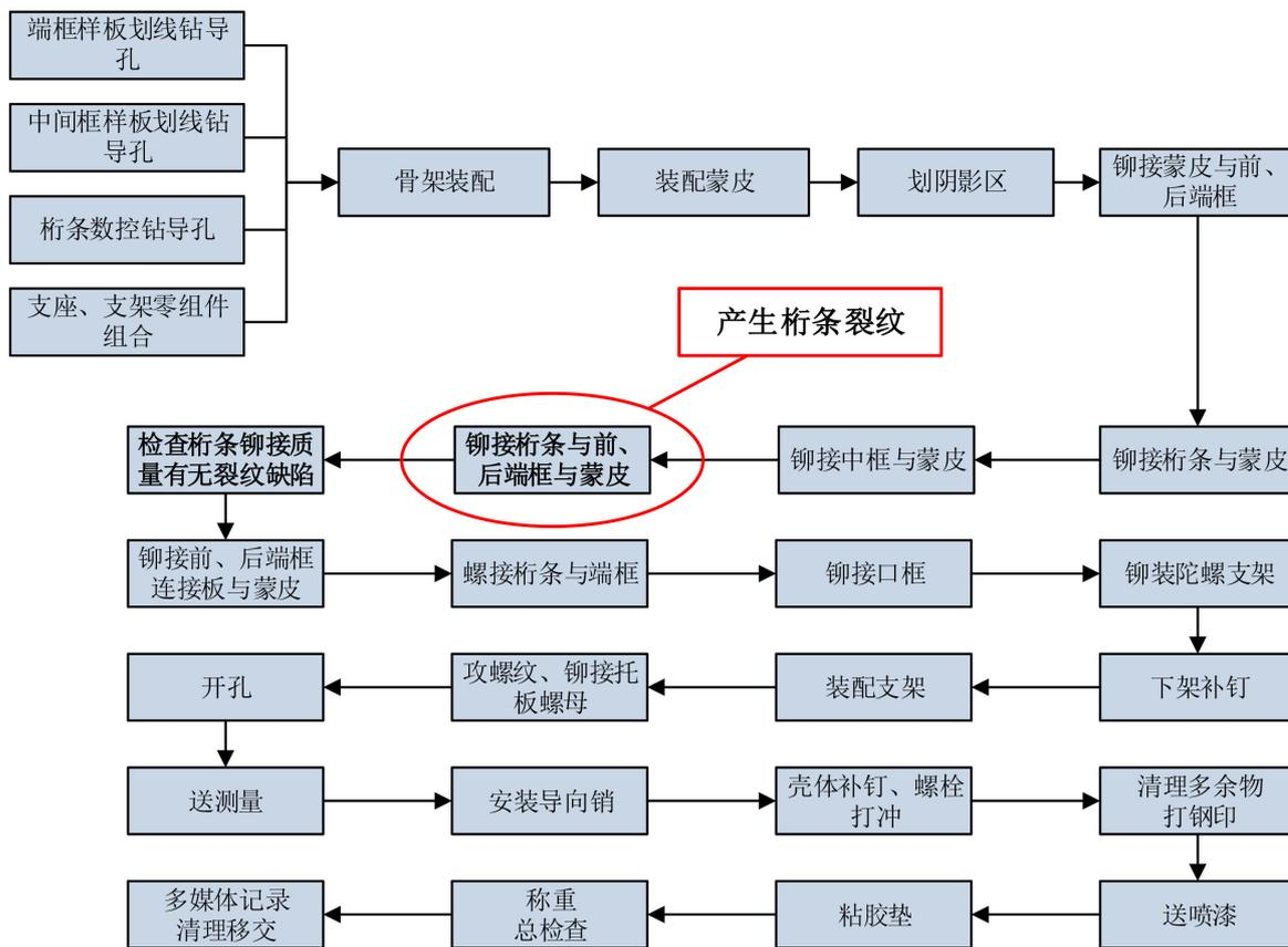
Figure 3. Process flow of Al-Li alloy strings riveting compartment assembly
