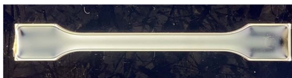
Figure 7. PMMA spline front stress detection
