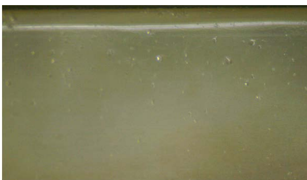
Figure 13. 300-fold microscope observation of polished parts
