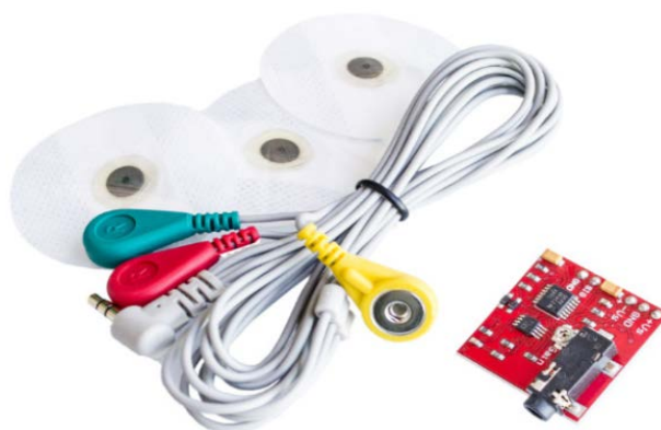
Figure 10. An electromyography acquisition device based on the surface electromyography signal principle
