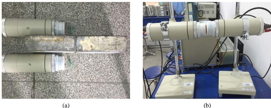
**Figure 3.** (a) The position of  $^{137}\text{Cs}$  with probe; (b) the position of  $^{60}\text{Co}$  with probe
