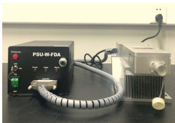
Figure 1. The image of 266 nm ceramic ultraviolet laser device
