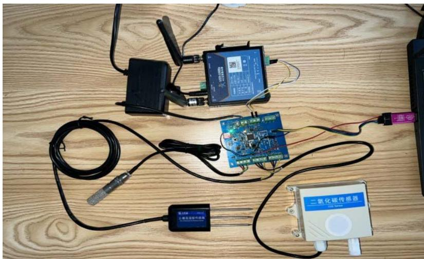
Figure 10. Equipment connection diagram of the edible fungus cultivation environment monitoring system
