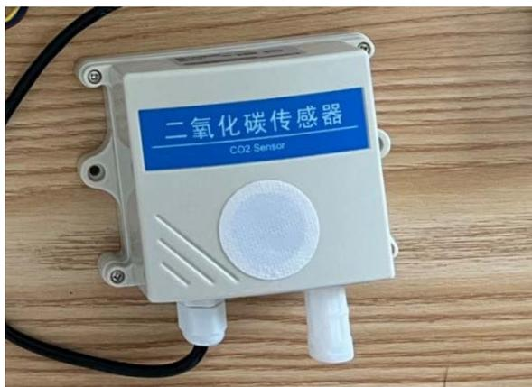
Figure 6. Carbon dioxide concentration detection module
