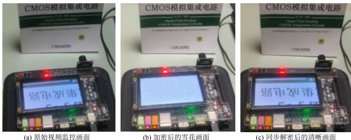
Figure 5. Real-time video encryption and decryption hardware test results 图 5. 实时视频加解密硬件测试效果
