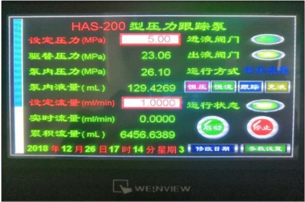
Figure 2. CYQ-III data acquisition control system touch screen interface
