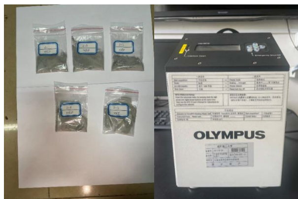
Figure 1. Sample after rock fragmentation (left) and X-ray diffraction analyzer (right) 图 1. 岩石破碎后样本(左)与 X 衍射实验分析仪(右)
