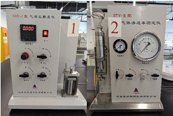
Figure 2. Gas porosity meter (left) and gas permeability meter (right) 图 2. 气测孔隙度仪(左)与气体渗透率测定仪(右)
