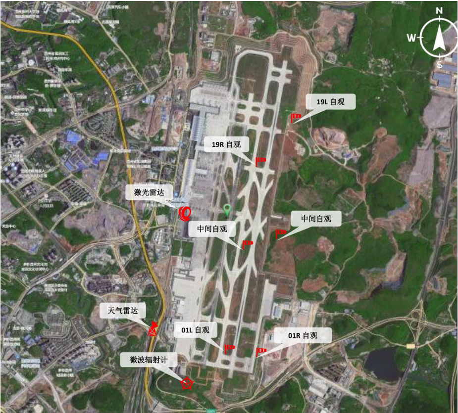
Figure 1. Location map of detection equipment at Guiyang Airport 图 1. 贵阳机场探测设备位置图
