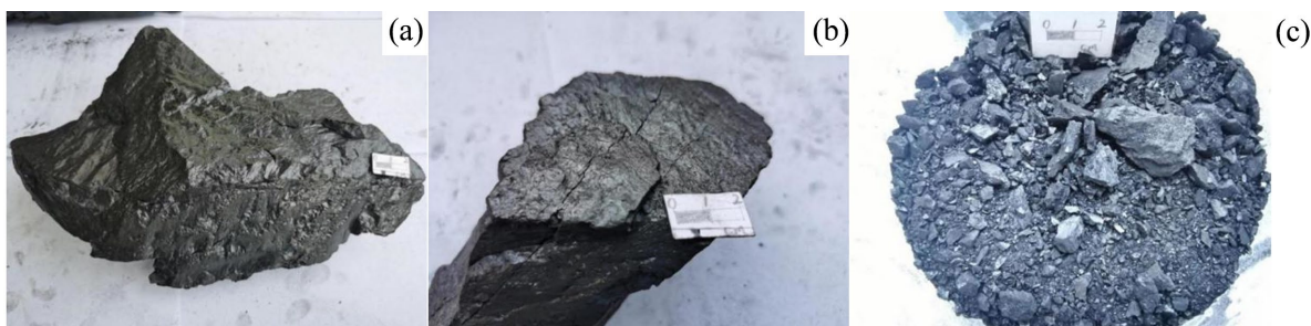
Figure 2. Macroscopic deformation characteristics of primary tectonic coal, fragmented coal and crushed coal 图 2. 原生构造煤、碎裂煤和碎粒煤宏观变形特征
