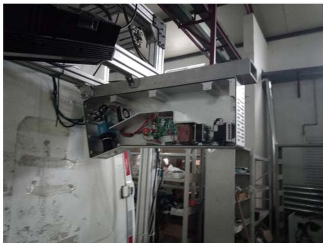
**Figure 2.** Three-dimensional acquisition equipment and components installed on test vehicle
