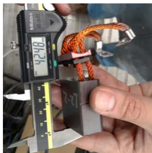
Figure 4. Measurement of carbon brush length
