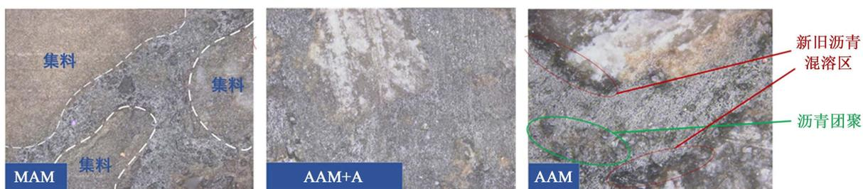
Figure 6. Miscibility morphology of asphalt mortar
