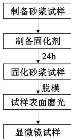
Figure 5. Sample preparation for microscope
