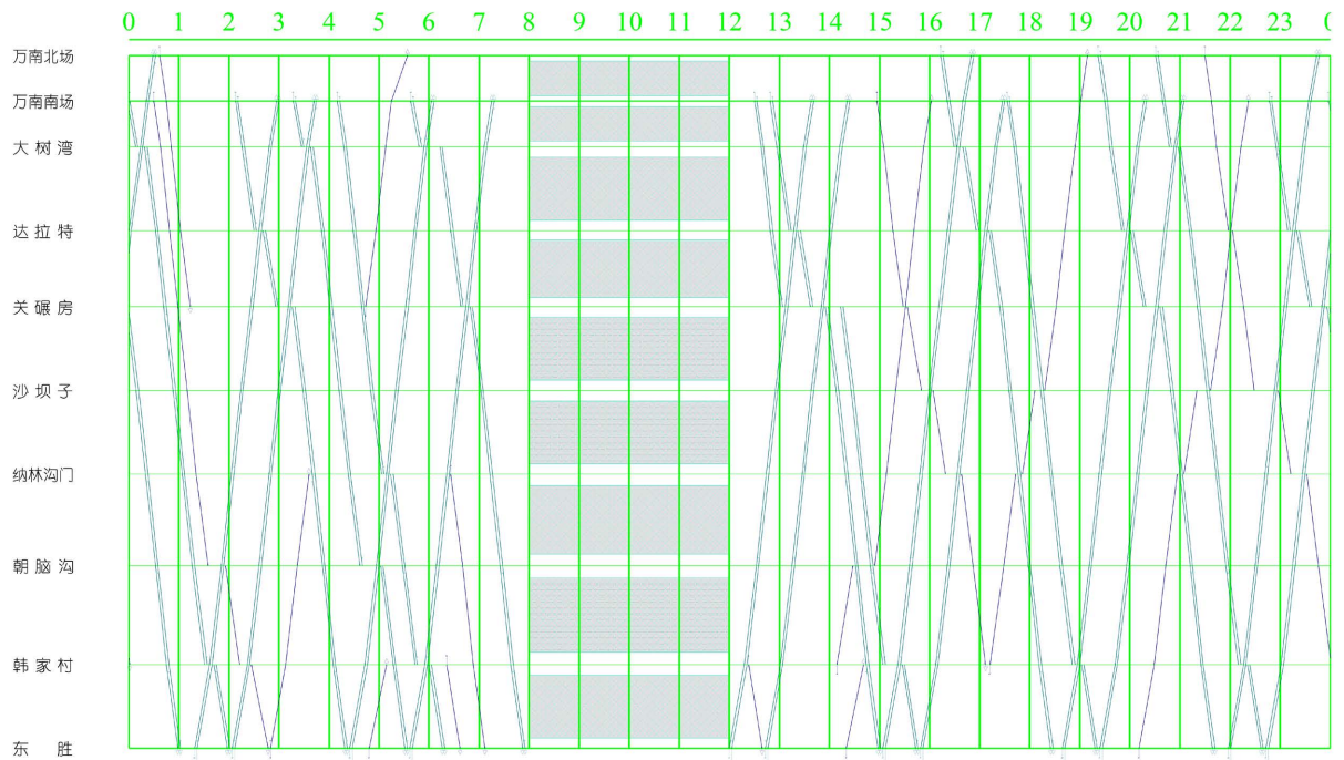
Figure 3. Diagram of train operations on the North Baotou-Shenmu Line in group mode 图 3. 群组模式下包神北线重载列车运行图
