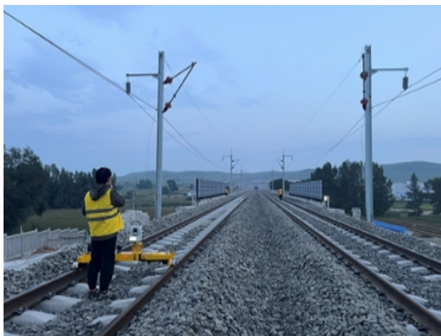
Figure 5. Diagram of the inertial navigation cart experiment
