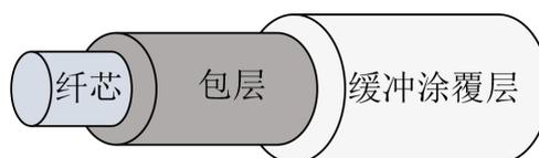
Figure 1. Structure of optical fiber
