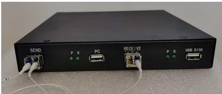
Figure 6. Photograph of unidirectional data transmission device
