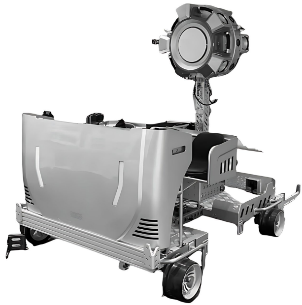
Figure 2. Specialized vehicles equipped with laser scanners 图 2. 专用车辆搭载激光扫描仪
