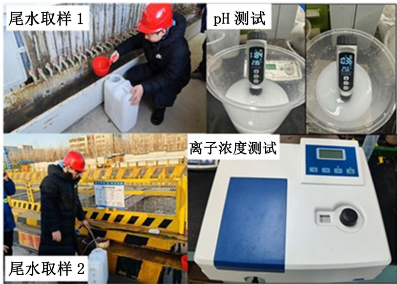
Figure 2. Property test of the tail water 图 2. 尾水性质测试
