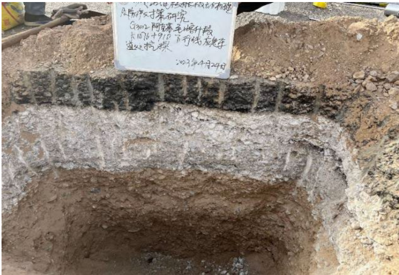
Figure 4. Trenching investigation results along the Aksu-Kashgar section of the G3012 Expressway 图 4. G3012 阿克苏至喀什高速公路挖探情况
