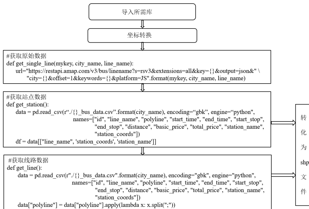
Figure 2. The process of obtaining public transportation data
