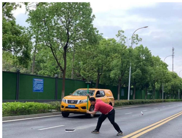
Figure 12. The heavy hammer strike for energy input 图 12. 能量输入的重锤敲击
