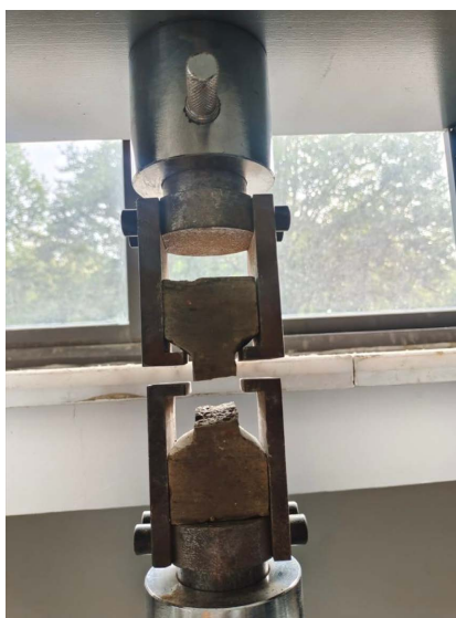
Figure 2. Loading device and specimen for uniaxial tensile test of solidified soil 图 2. 固化土单轴拉伸试验加载装置及试件
