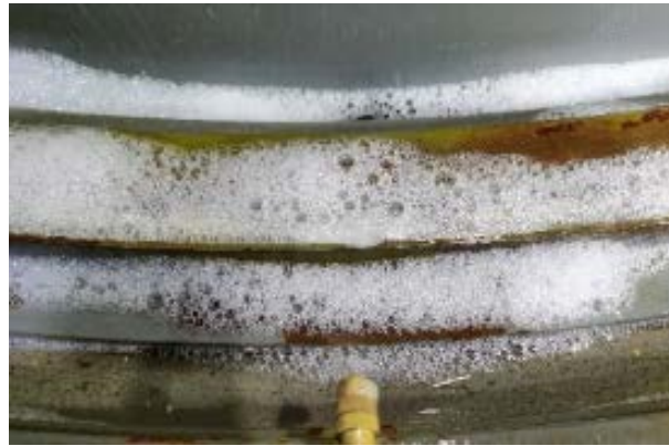
Figure 2. Spraying anti-wear fluid medium on the rail surface 图 2. 轨面上喷洒减磨液介质
